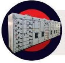
Power Control Centers are used for distribution and control of power with protection of power source and equipments from short circuit, overload, earth fault, under and/or over voltage etc. The fault levels areas as high as 50KA or 65KA for 1 second. The approriate bus bar system are incorporated to suit the fault level as well as to restrict temprerature rise above ambient
